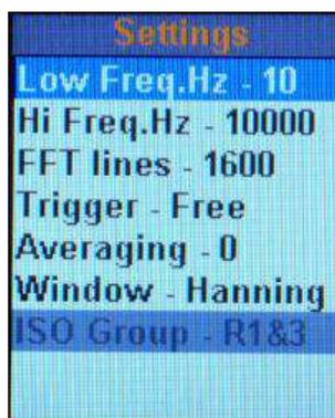
**Low Freq** – lower frequency limit. Can be set to 1, 2, 10 Hz.
