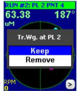
The analyzer displays calculated corrective weights that need to be attached to planes №1 and №2 to correct the imbalance.
