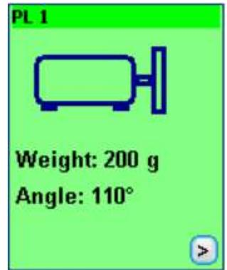
Press the button
