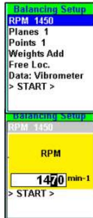
If the actual speed and the speed set in the balancing parameters differ by more than 5%, the device will display an error message during the measurement
