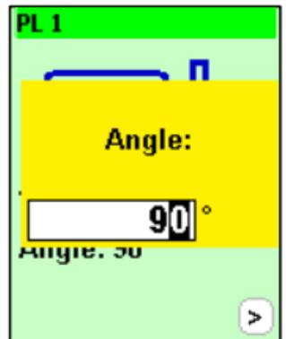
Start the machine and measure the vibration levels at all four points with the test weight attached to plane #1.
