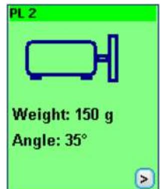
Start the machine and measure the vibration levels at all four points with a test weight attached to plane № 2
