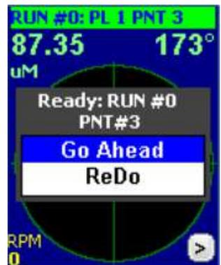
Place accelerometer at measurement point #4.
