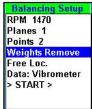
Correction masses can be attached in any angular position - Free Loc. Or in fixed places (for example, on fan blades). The number of fixed seats can be set from 3 to 18 seats.
