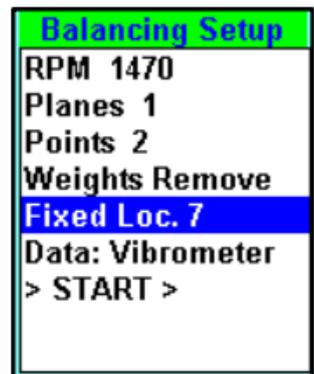
The balancing program implies that the angles (and the fixed numbering of places) are always calculated against the direction of rotation of the machine!
