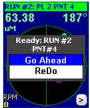
Stop the machine. Choose whether to keep or remove the trial weight on plane №2.
