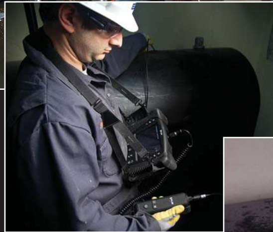
Checking aircraft engines and airframes for cracks, wear, defects and debris; Inspecting oil tank for corrosion
