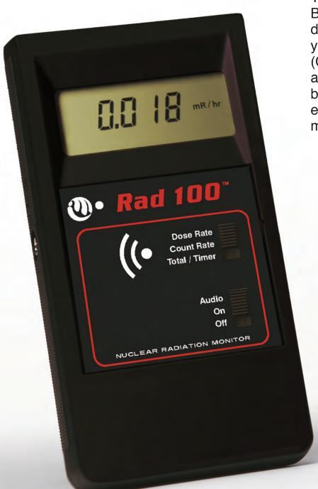
The Rad 100<sup>™</sup> measures Alpha, Beta, Gamma, and X-radiation. Its digital display shows readings in your choice of counts per minute (CPM), µSv/hr or mR/hr, or in accumulated counts. A red LED blinks and a beeper chirps with each count (the chirp can be muted).
